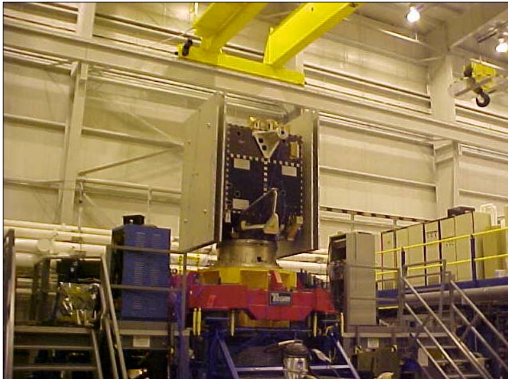
Figure 7. Science mission spacecraft qualification primary structure with mass simulators undergoing vertical vibration test on new guided head expander.
