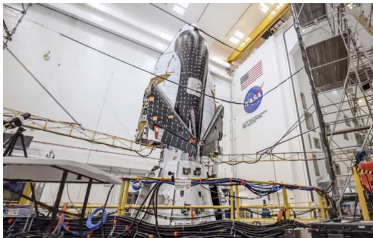
The Sierra Space Dream Chaser Spaceplane undergoes swept sine testing.
