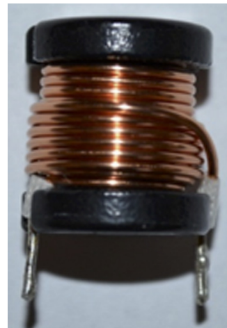
Fig. 5 Inductor with tape wrap removed
