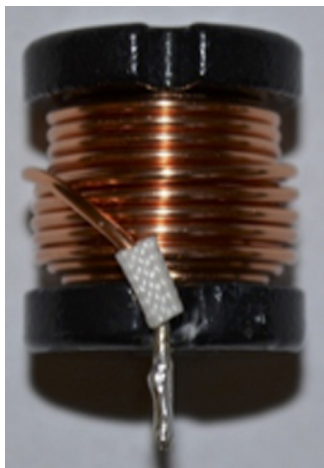
Fig. 7 Outside coil wrap (stiff lead)
