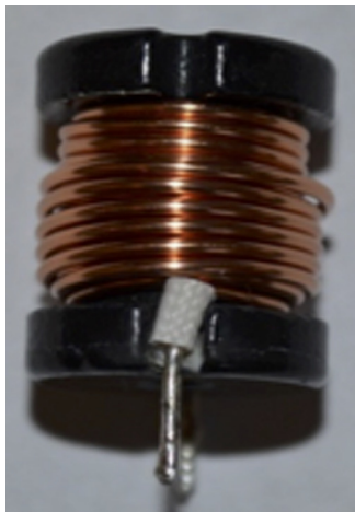
Fig. 8 Inside coil wrap (compliant lead)
