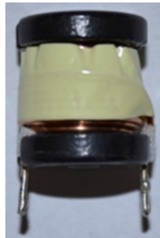
Fig. 4 Inductor with shrink wrap removed
